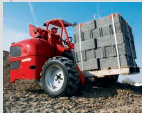
With a 50 HP Perkins engine connected to its 3 driving wheels, the TMT 2520 SR has more power to be at ease on any kind of ground.
