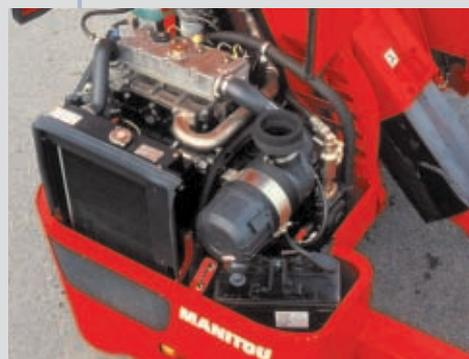
With a 50 HP Perkins engine connected to its 3 driving wheels, the TMT 2520 C has more power to be at ease on any kind of ground.
