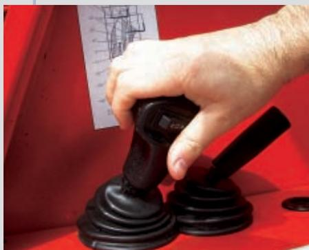
This new « boom control » joystick now integrates the « reversing shift » function : the driver can keep one hand on the steering wheel and one hand on this joystick to operate any movement. Time saving and much better driving position.
