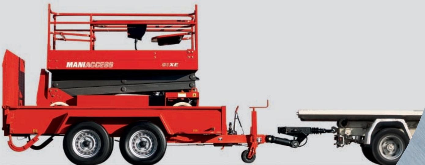
These very light machines can be transported easily on trailers with a maximum weight of 3.5 t.
