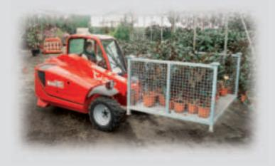
Rough terrain With its 3-wheel drive, its differential lock and its ground clearance, Twisco can cross all obstacles.
