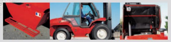
The cab is suspended to insulate the operator from vibrations and noise.
