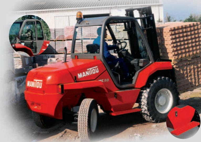
Standard fittings on the MC 30 include a left-hand exterior rear-view mirror, reversing shift on the steering column and control levers in line near the seat. MANITOU also offers a wide choice of masts that allow total vision. The front axle of the MC 30 has a multidisc oil immersed brakes and hydraulic differential lock. The integral steering ram on the rear axle gives a very short turning radius for yard work.
